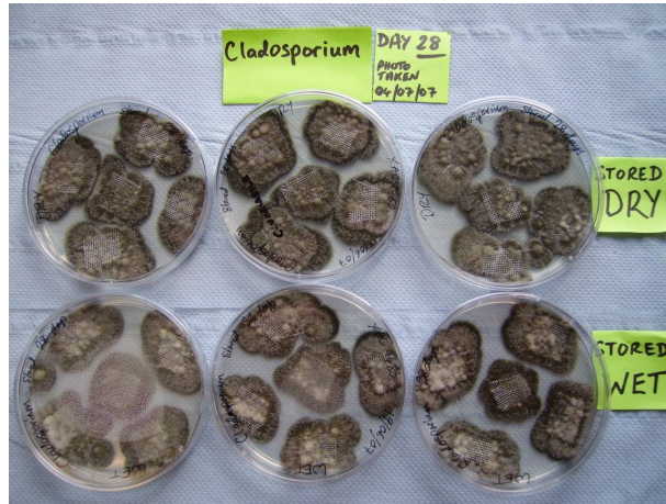
Figure 2. Growth of Cladosporium variabile from mesh pieces after 28 days storage under wet and dry storage regimes
